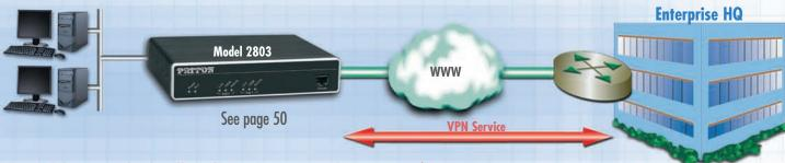
The Model 2800 Series is a line of IPSec/VPN Enterprise Routers with strong encryption and a variety of integrated WAN interface options.
